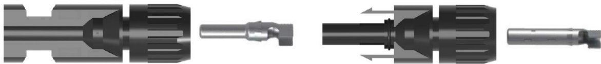
Negative Coupler & Contactor Pin Positive Coupler & Contactor Pin. FIG. 7-9 Structure Illustration of DC Connector
