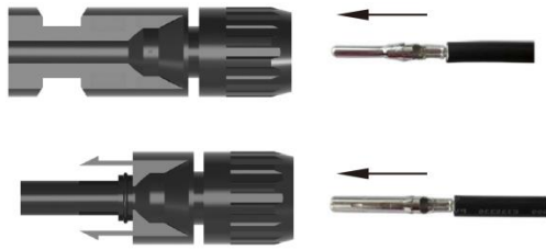
FIG. 7-12 Insert the Contact
