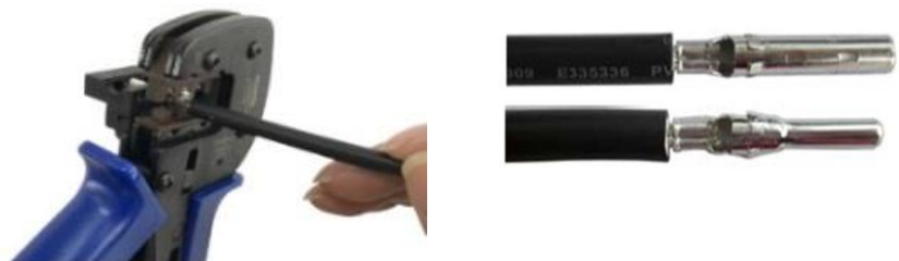
FIG. 7-11 Crimp the Contact
