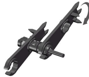
FIG. 7-13 Tighten the Cable Gland
