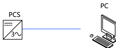
Fig3-4 Ethernet communication for a single PCS
