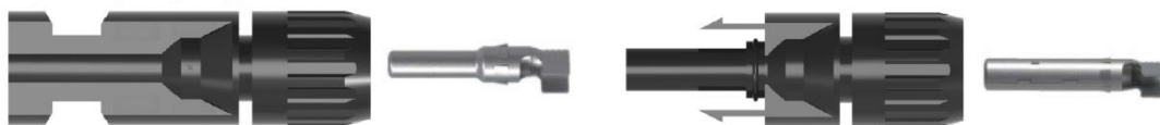
Negative Coupler & Contactor Pin Positive Coupler & Contactor Pin. FIG. 7-10 Structure Illustration of DC Connector
