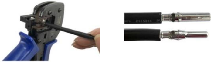
FIG. 7-12 Crimp the Contact
