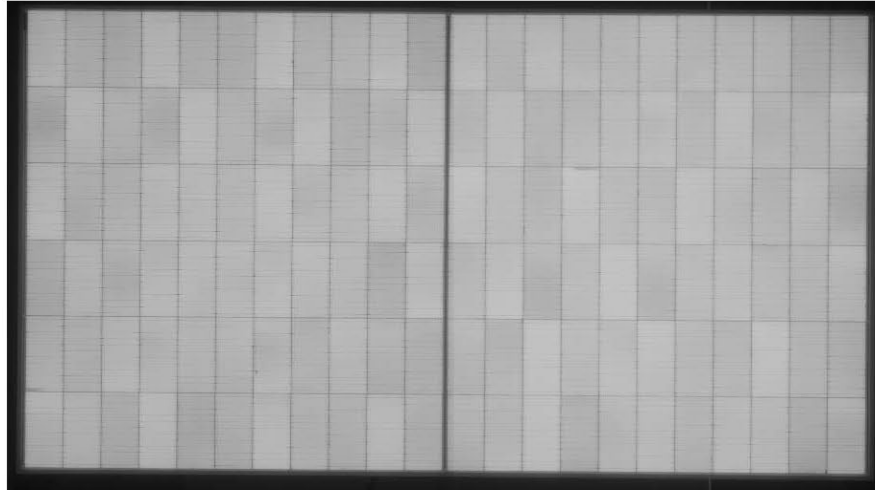
Figure 17 Initial EL image of sample No. 6131138-4
