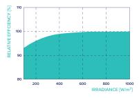
Typical module performance under low irradiance conditions in comparison to STC conditions (25 °C, 1000 W/m<sup>2</sup>).
